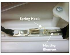
Step 3. Remove Heating Elements. Removing the heating element may be a bit tricky and requires some patience. Using either your fingers or a pair of small pliers, pull the spring hook from the hole of the heating element. When you release one end of the element from the spring hook, the other end will release easily.
