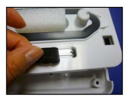
Step 2. Remove PTFE Adhesive. Open the upper jaw of the vacuum sealer and gently peel the PTFE adhesive (sealing strip) from the heating element. You may have to push some of the PTFE adhesive through from the lower base.
